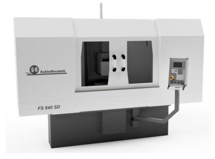
This machine was conceived especially for individual and small-lot production. In a workshop, it is necessary that surface grinding machines are easy to use. Process modifications must be easily realisable. The SD-control was developed for this scope of operations. Especially for adjustment work, the infeed can be made with  $\mu m$ -precision by means of the electric manual wheel – analogue to the manual wheel of a hand-controlled machine.
