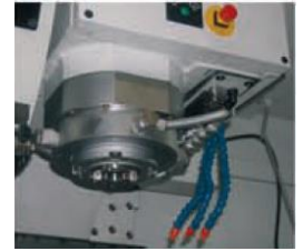
water curtain around spindle
