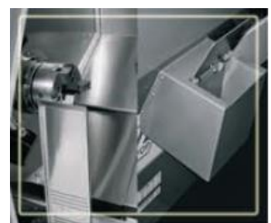
Cut off parts catcher for automatic parts collection
