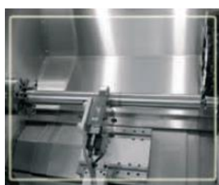
Hydraulic steady rest for long rods and shafts
